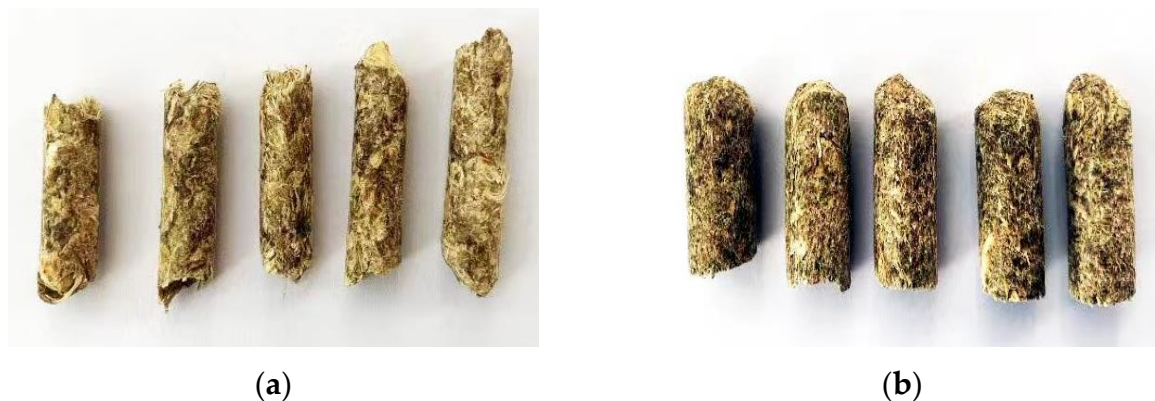
Figure 1. Caragana korshinskii pellet. (a) 5 mm particle size; (b) 9 mm particle size.
