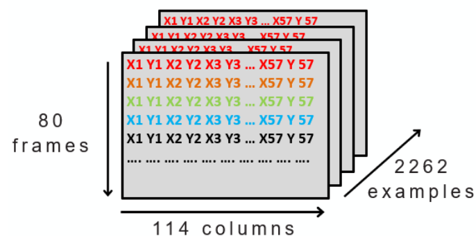
Figure 6. Representation of the decoder input format (different colors for each frame landmarks).
