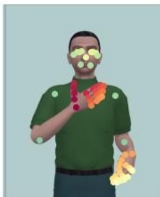
Figure 3. Landmarks over a frame from the sign “AMO” performed by one of the avatars (red landmarks are related to right hand, orange and yellow ones are related to the left hand, and green ones are related to the body).
