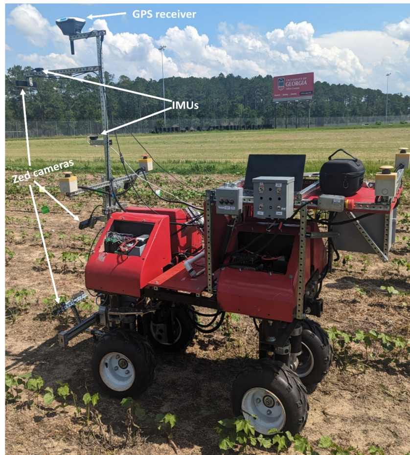
Figure 2. Front view of the rover deployed to collect video streams of cotton plants in Tifton, GA.
