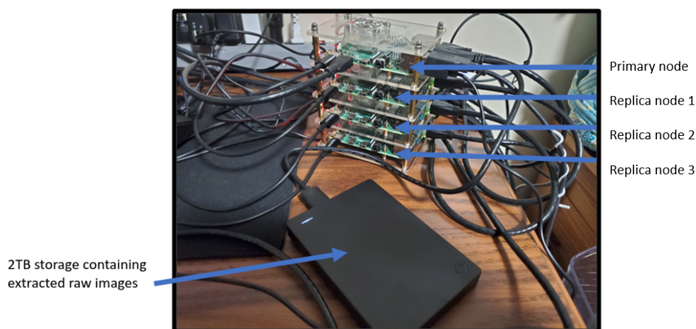
Figure 8. A closeup of our distributed computing cluster setup with four nodes.
