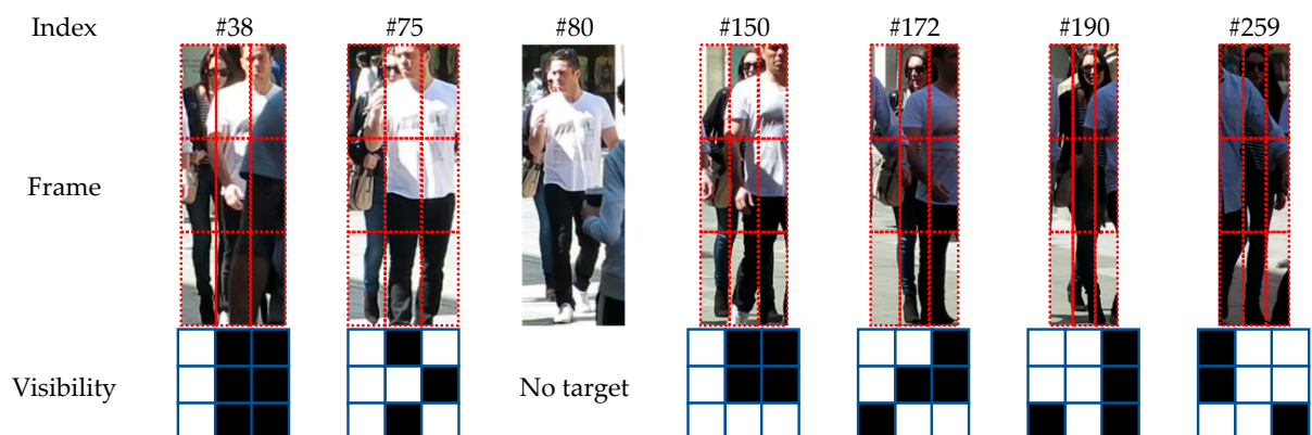
Figure 5. Example of detecting and tracking of a frequently occluded target. The visibility map shows the visible parts of the lady behind the man in white.
