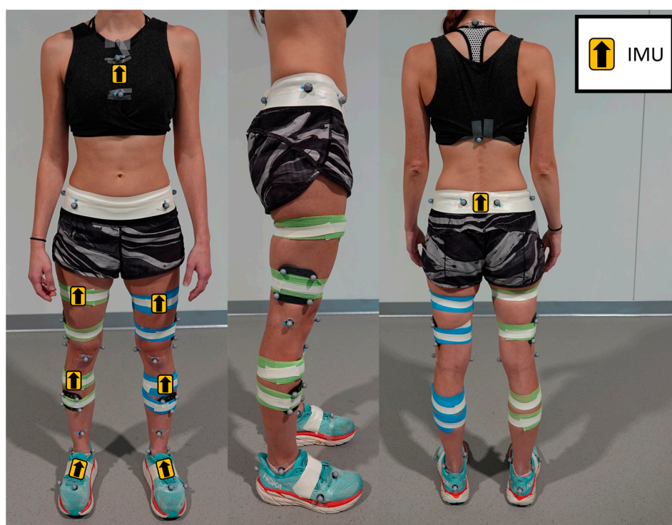
Figure 1. Placement of eight Delsys Trigno Avanti IMU sensors: sternum, sacrum, anterior thighs, anterior shanks, and the dorsal side of the feet. Retroreflective markers are placed on bony landmarks based on a modified Cleveland Clinic marker set [30].
