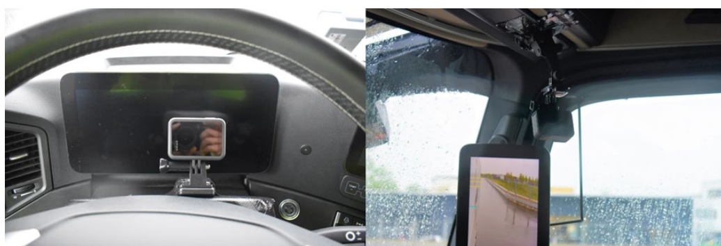
Figure 6. Mounting action cameras to record instrument cluster display and mirror fields of view.
