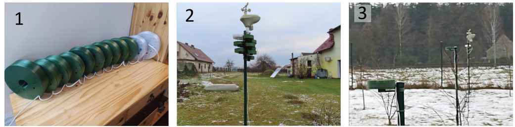
Figure 6. PM sensors at the different research conditions. (1) Condition a: Tests of the sensors in the building; (2) Condition b: Measurements with Sensors A–J at Location A; (3) Condition c: Measurements with Sensors C1–C3, D, and E at Locations C, D, and E (other sensors not shown in the photo).
