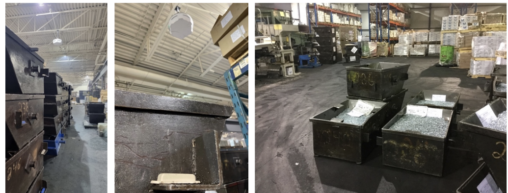
ATR700 RFID over stacked buckets equipped with tags
