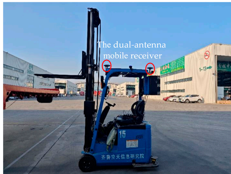
Figure 9. Diagram of the dual-antenna mobile receiver installation locations.
