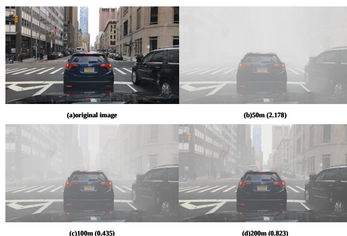
Figure 8. Simulated fog images with scores at three different densities and examples of clear images, with fog thickness decreasing as visibility increases.
