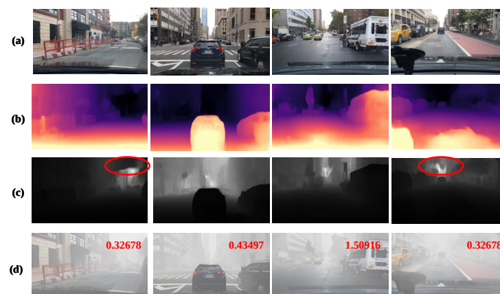
Figure 7. Examples of depth estimation and foggy image synthesis, (a) original images from BDD100K, (b) relative depth maps predicted by Monodepth2, (c) absolute depth maps obtained by dense geometric constraints, and (d) synthetic fog (evaluation of the corresponding fog image in the upper right corner of the image).
