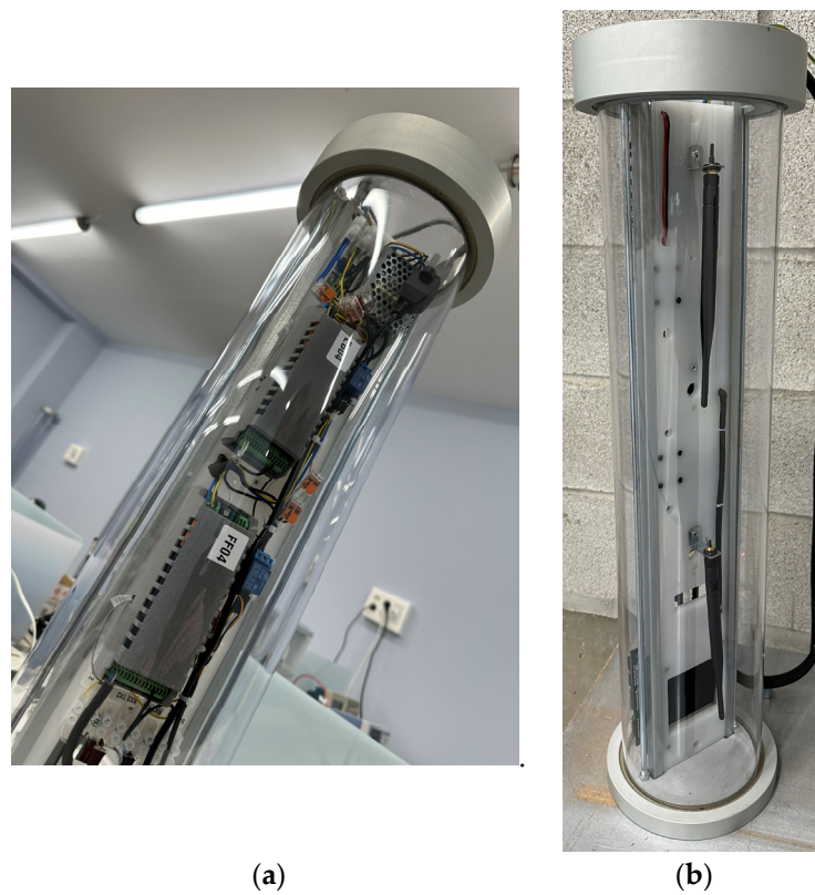
Figure 22. Images of the gateway: (a) the side where two PCBs are placed; and (b) opposite side: two LoRa antennas.
