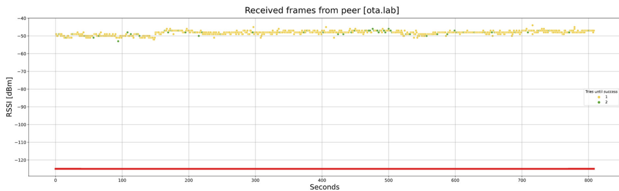
Figure 24. Unicast OTA procedure, with a distance of 2 m and no obstacles: RSSI of each frame. The red line corresponds to the sensitivity of the receiver.
