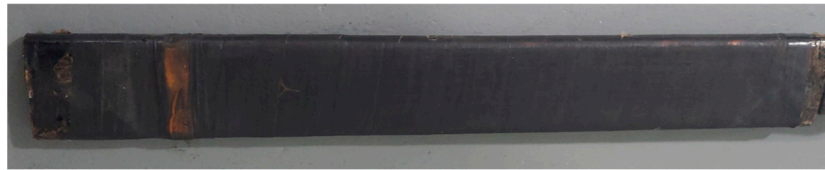
Figure 9. Photograph of the hydrogenerator bar.
