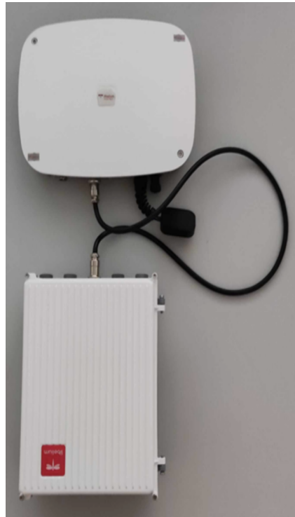
Figure 5. Smart Spot—IOT device for environmental parameter sensing.
