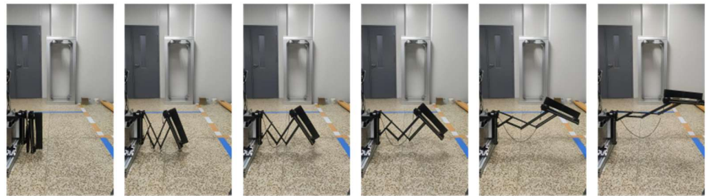
Figure 21. The experimental process of the radial deployable mechanism.
