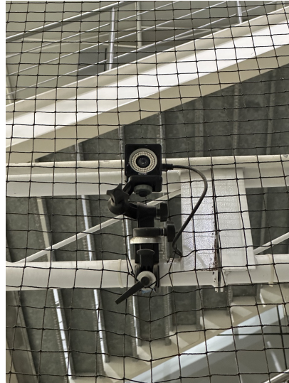
Figure 5. OptiTrack Prime 13 camera from the OptiTrack-Motive Motion Capture system.
