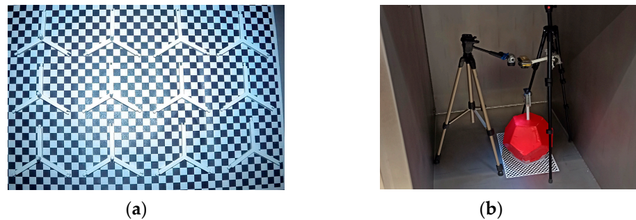
Figure 4. The 3D-printed parts (a) and the whole dodecahedron formed structure (b) inside the low air pressure chamber.
