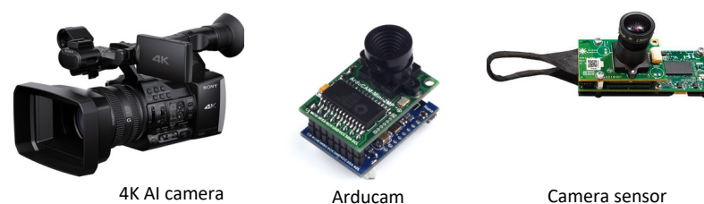
Figure 10. Some example devices of cameras technologies used for occupancy detection, estimation, and prediction.
