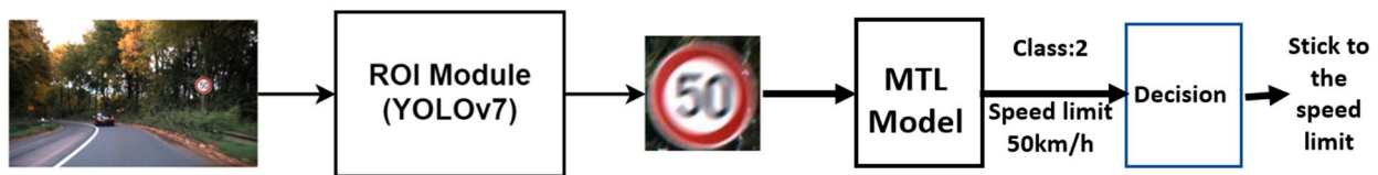
Figure 7. Different blocks of the system: the ROI module, the classification MTL model, and the decision model.
