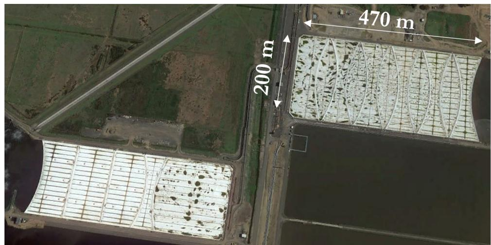
**Figure 1.** Anaerobic lagoons at the WTP.
