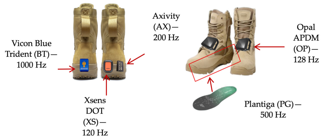
Figure 2. Schematic of sensor positions on/in military boots.
