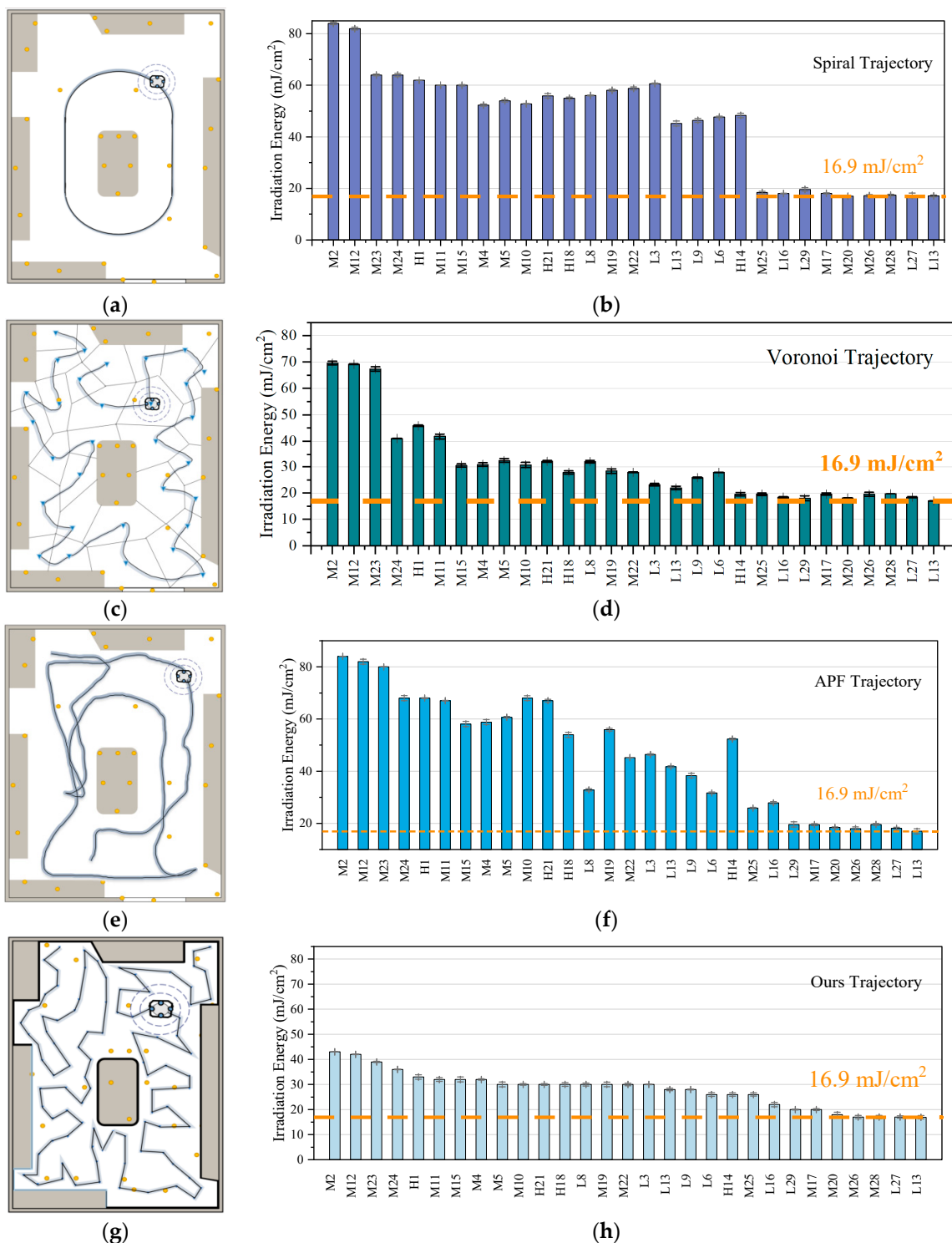
Figure 13. Comparative experiment: The experiment compared the dose coverage effect after executing four path algorithms. (a,b) Spiral. (c,d) Voronoi. (e,f) APF. (g,h) Ours. The illumination energy measurement device was deployed at the observation points in Figure 8d, and the robot executed the trajectory according to the algorithm in the left figure. After the disinfection, the distribution of UVC dose at each point was measured as shown in the right figure. For easy comparison, the abscissa adopts a unified labeling order, and the ordinate adopts a proportional scale.
