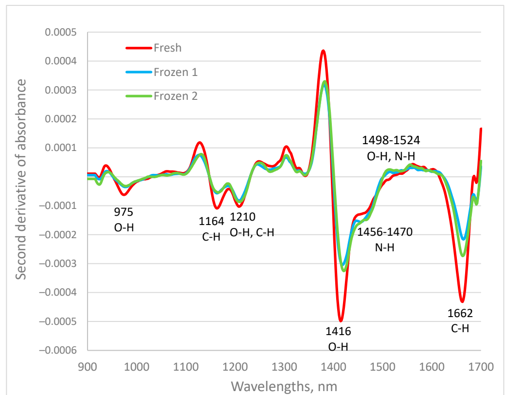
Figure 2. The second derivative of spectra of one fish sample from the ventral region, measured fresh, after the first freezing and thawing, and again after the second freezing and thawing.
