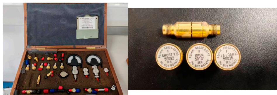
Figure 6. Calibration kit 80858B was used in this study.
