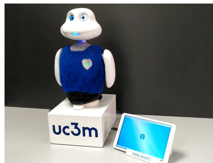
Figure 1. Mini, a social robot developed for interacting with adults who are older that suffer from mild cases of cognitive impairment.
