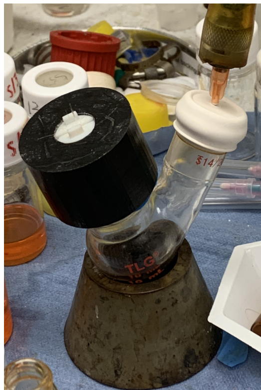
Figure 11. Two-neck flask setup consisting of a nitrogen line connected to a syringe needle inserted into a septum on the angled neck. The nanomaterial was loaded into the flask. The septum was secured with super glue. The 3D-printed PCF loaded was inserted onto the vertical neck with one end of the PCF sitting within the nanomaterial solution. Fun-tak was used to create a better air seal around the bottom of the 3D-printed PCF loader.
