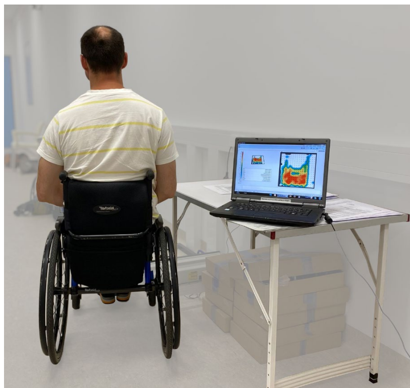
Figure 1. Example of a seat pressure measurement. Measurements were taken using a pressure mat (BodiTrak®) placed on the participants' own seat cushion in their own wheelchair.
