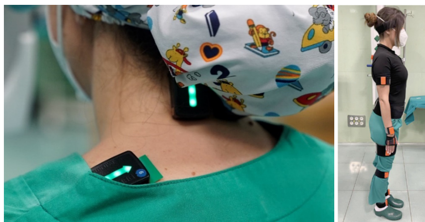
Figure 3. Example of location of EMG sensors (left) and inertial sensors for motion analysis (right).
