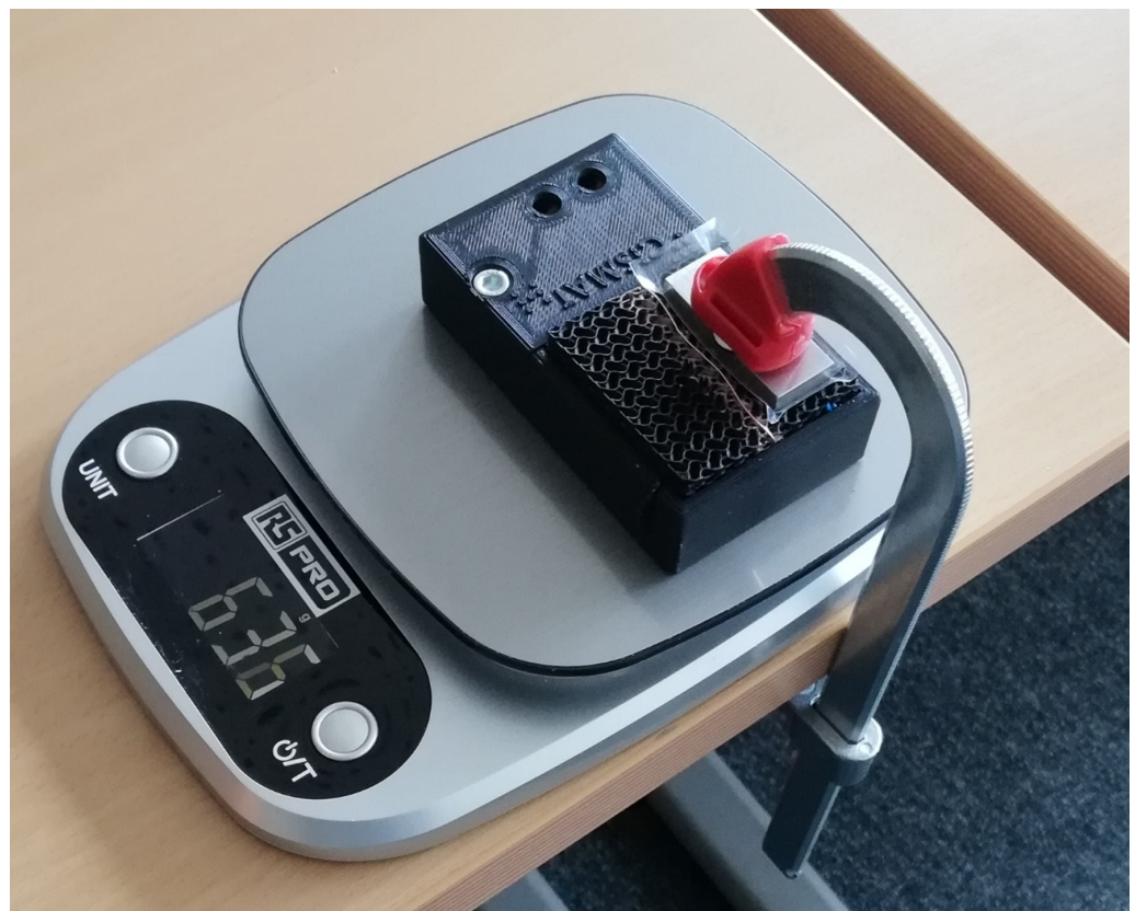
Figure 5. Test setup: structure in its frame connected to its electronics. It is positioned on a scale to measure the force applied by the clamp.
