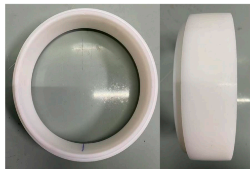
Figure 10. Scaled segment model fabricated by LDPE.
