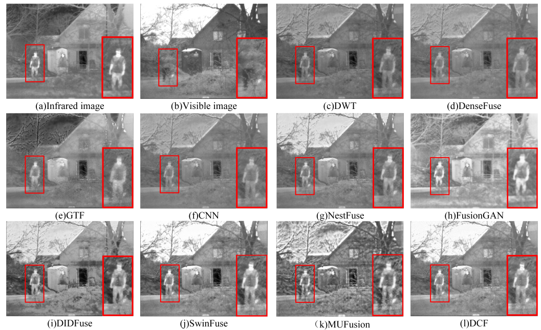
Figure 8. Fusion results of DCF with nine other fusion methods in the image soldier-behind-smoke-1. For a clear comparison, we selected a prominent region (i.e., the red box) in each image and zoomed in to facilitate a detailed demonstration of the differences in fusion effects.
