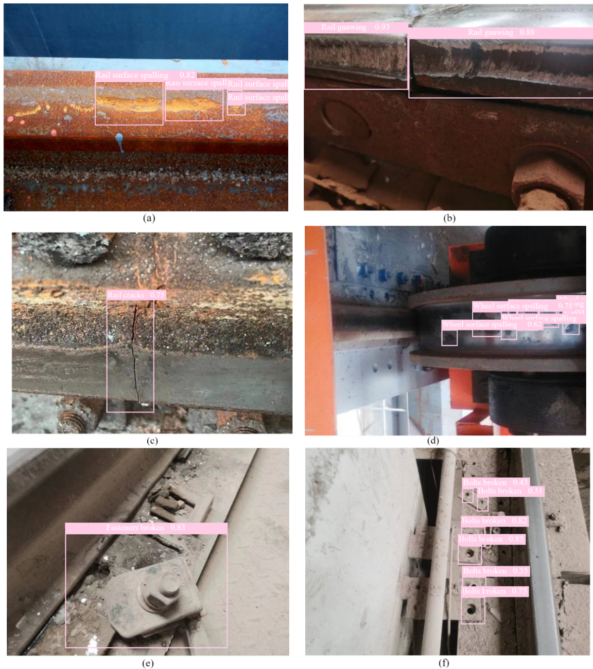
Figure 8. Detection results of the proposed method: (a) Rail surface spalling. (b) Rail gnawing. (c) Rail cracks. (d) Wheel surface spalling. (e) Fasteners broken. (f) Bolts broken.
