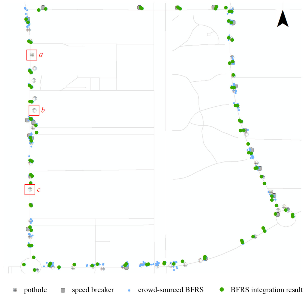
Figure 13. The road surface sensing result from crowd-sourced datasets. The red rectangles of a , b , c , refer to the undetected BFRS.
