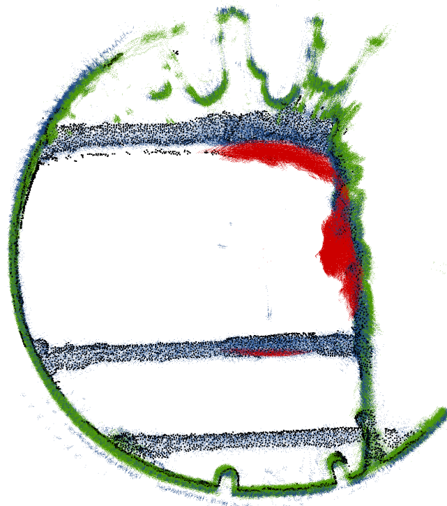
Figure 11. Horizontal cross-section of shaft. Red—Livox TELE-15, Blue—VLP-16, Green—VLP-32c. Black—FARO Focus 3D.
