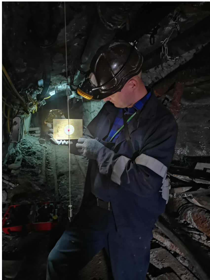
Figure 10. Pointing to the underground control point—showing the factors affecting the accuracy of determining the coordinates of the ground control points.
