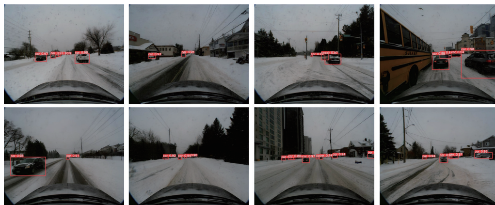
Figure 6. We present the 2D object-detection results of our algorithm on the validation set of the CADC public dataset. The red boxes indicate the target locations predicted by our algorithm, and the corresponding numbers represent the confidence scores (suggested to view in enlarged mode).
