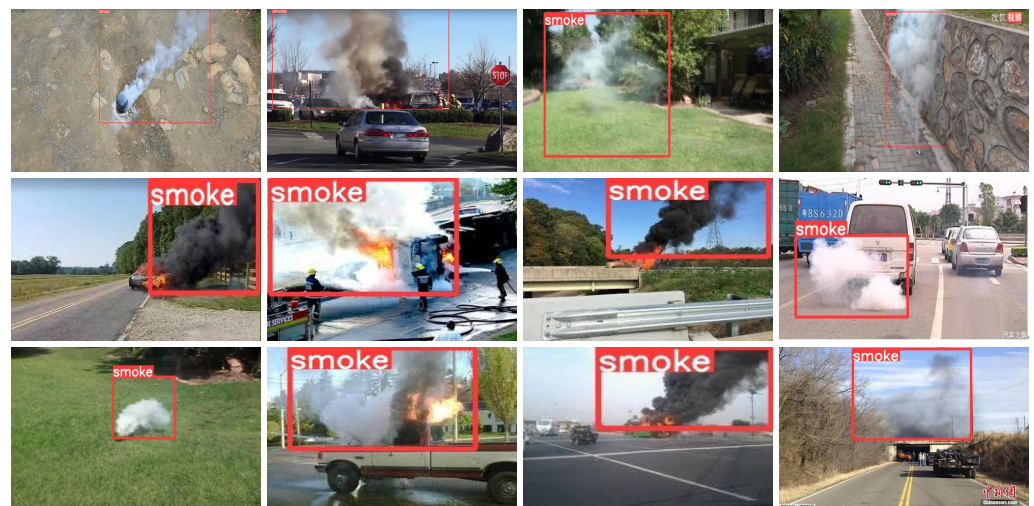
Figure 9. Visual detection for smoke images in the real application. These images are randomly downloaded from the Internet and untrained, and our CLSNet can still accurately monitor smoke.
