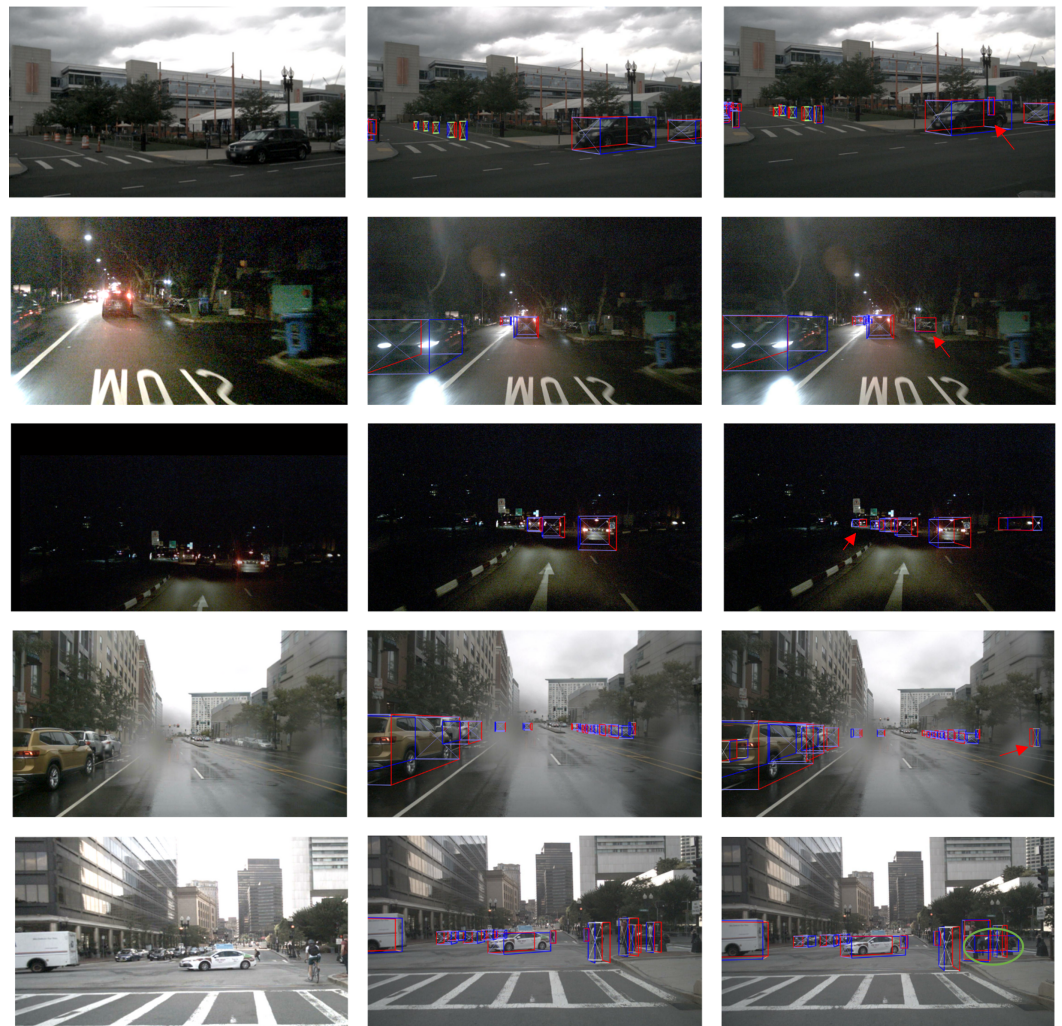
Figure 12. Qualitative comparison between our approach and CenterFusion under various scene conditions. For each row, the images from left to right are the raw image, the detection result of CenterFusion, and the result of our approach.
