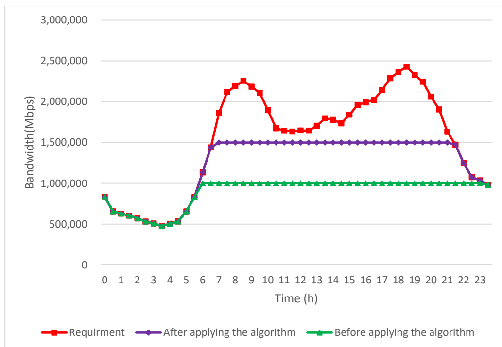
Figure 15. Contrast of bandwidth requirements and assigned bandwidth before and after algorithm implementation.
