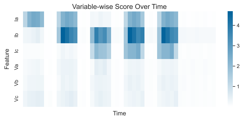
Figure 9. Aggregated variable-wise scores for all features across all timestamps, with bins of width \Delta t = 250 .
