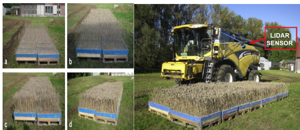
Figure 16. Different crop densities and combine harvester with LiDAR system (a) 100 ears per \text{m}^2 ; (b) 200 ears per \text{m}^2 ; (c) 300 ears per \text{m}^2 ; (d) 400 ears per \text{m}^2 [194].
