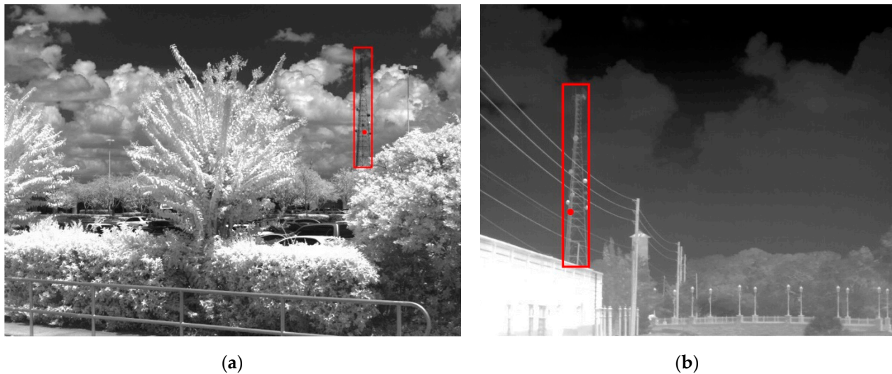
Figure 3. Image in NIR (a) and LWIR (b) of the same tower taken at different locations and target ranges. In NIR, the tower is dark under a bright background, whereas in LWIR, the tower is bright under a dark background. Each participant's response is represented by a red dot. In the above cases, both dots lie within the rectangular ground truth bounding box and are counted as a correct detection.
