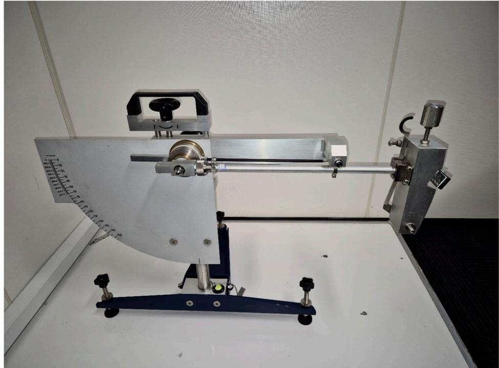
Figure 4. British Pendulum machine.
