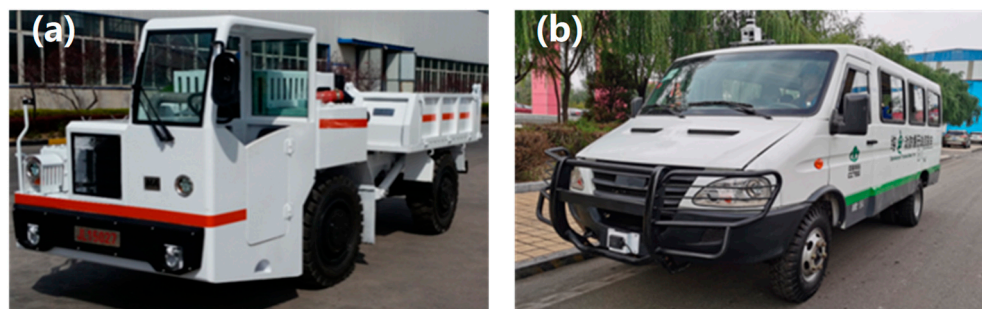
Figure 1. Explosion-proof rubber-wheeled vehicles manufactured by China Coal Technology & Engineering Group, Taiyuan Research Institute. (a) A traditional explosion-proof rubber-wheeled vehicle for material transport; (b) an autonomous driving prototype of an underground coal mine transport vehicle.
