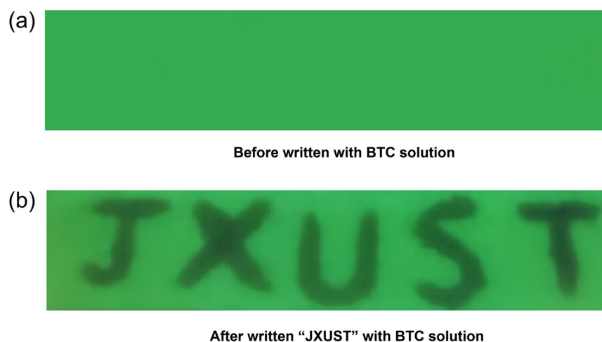
Figure 5. Fluorescence changes of BDTA test strip without (a) and with (b) 10 mM BTC solution.
