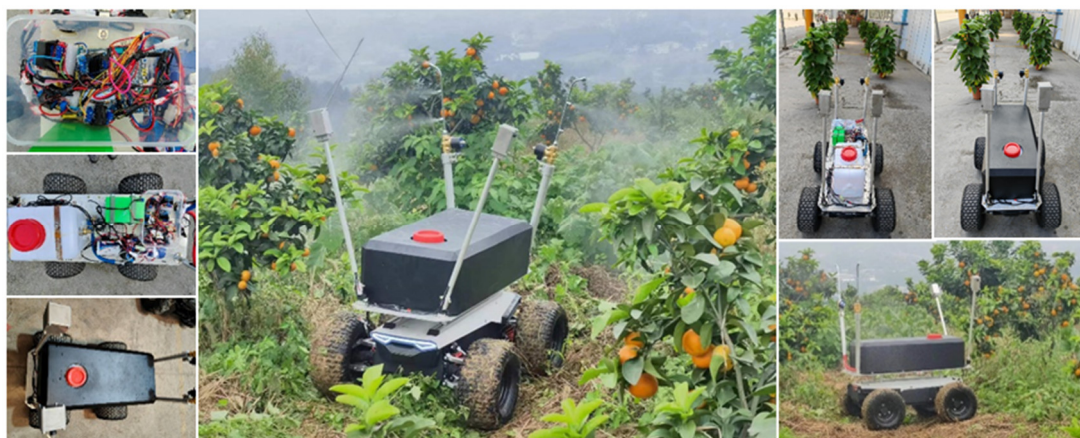
Figure 8. Orchard disease detection device used for disease data collection.
