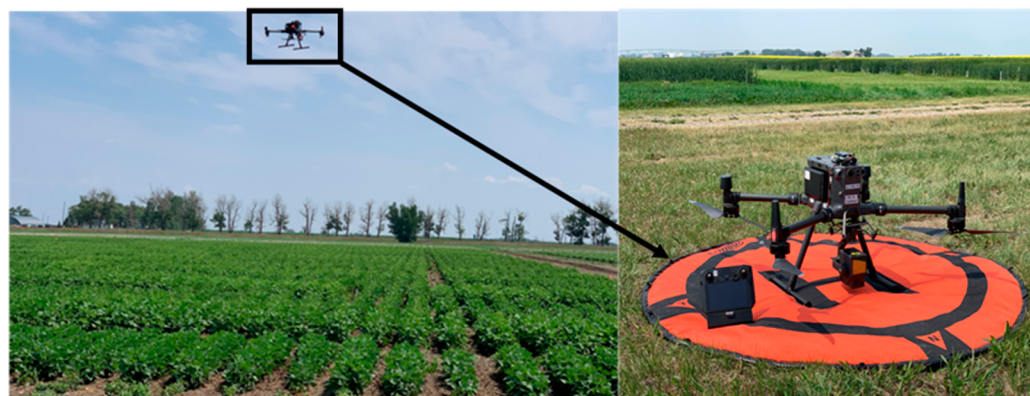
Figure 1. UAV flying over the dry bean plots (left) and UAV system with the LiDAR sensor (right).
