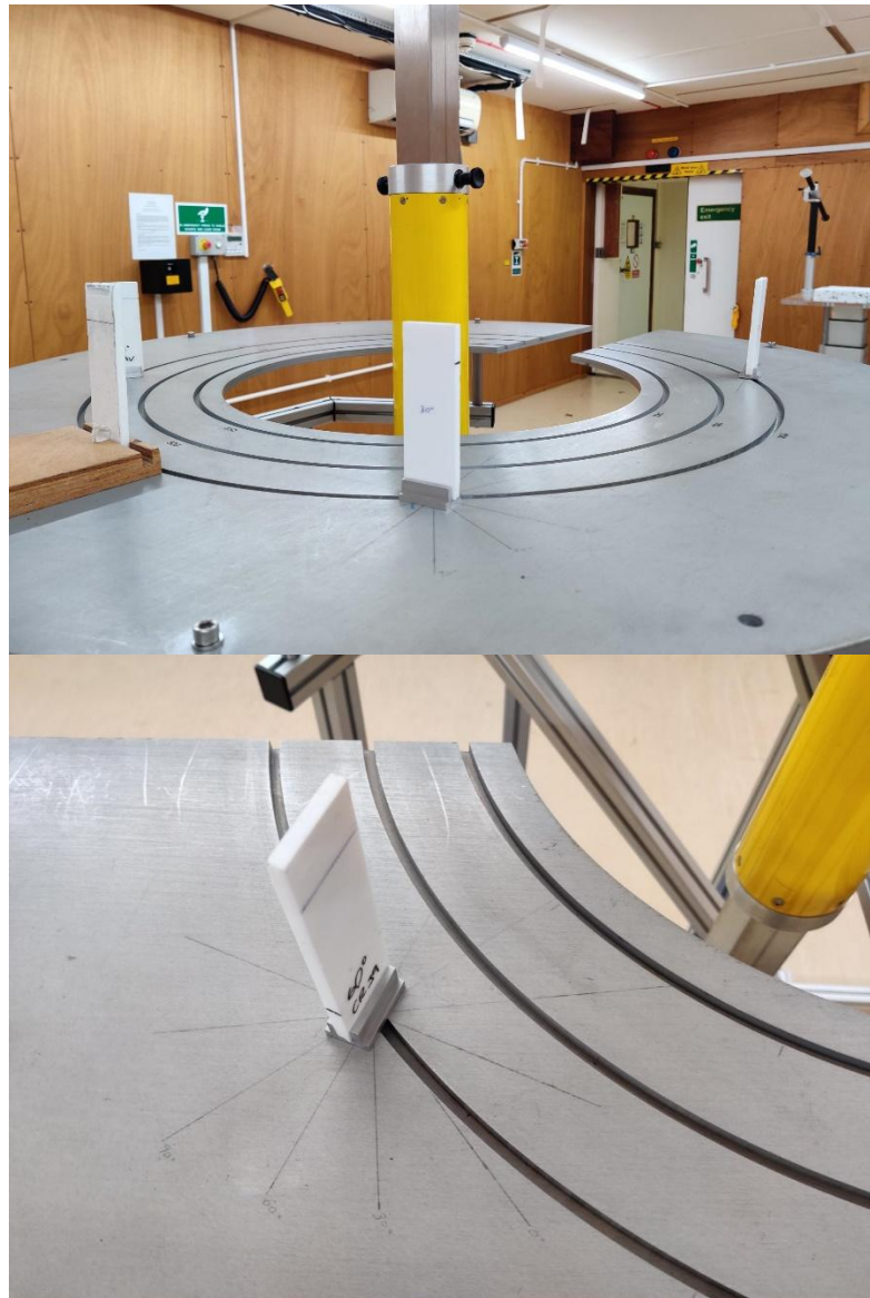
Figure 1. Diagrammatic and photographic explanation of the experimental set up at the UKHSA. Note that in this experiment, we compared standard CR39 detectors at 0°, 30°, and 60° angles to the source with alternative detectors (RAV) with a different plastic formulation. We do not report on the latter in this paper.
