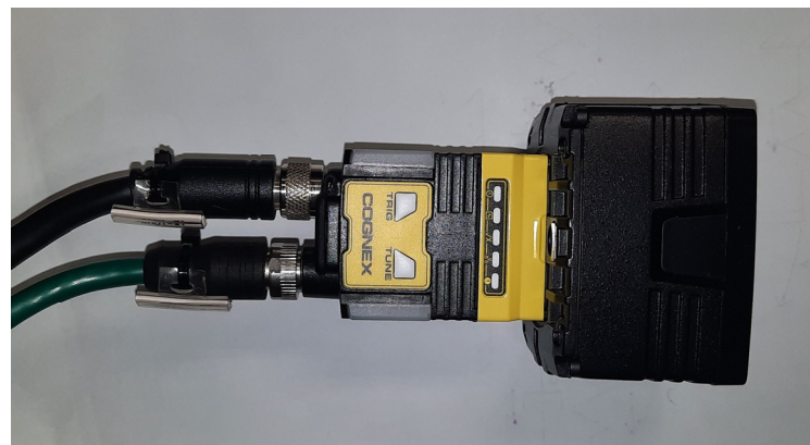
Figure 1. Cognex In-Sight 2802C camera used in the study.
