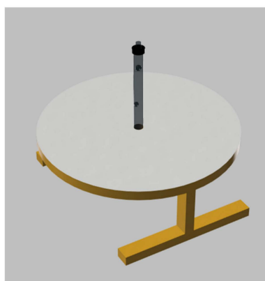
Figure 14. 3D-printed fixture with LED light source used for positioning and illuminating fiber optic tubes.
