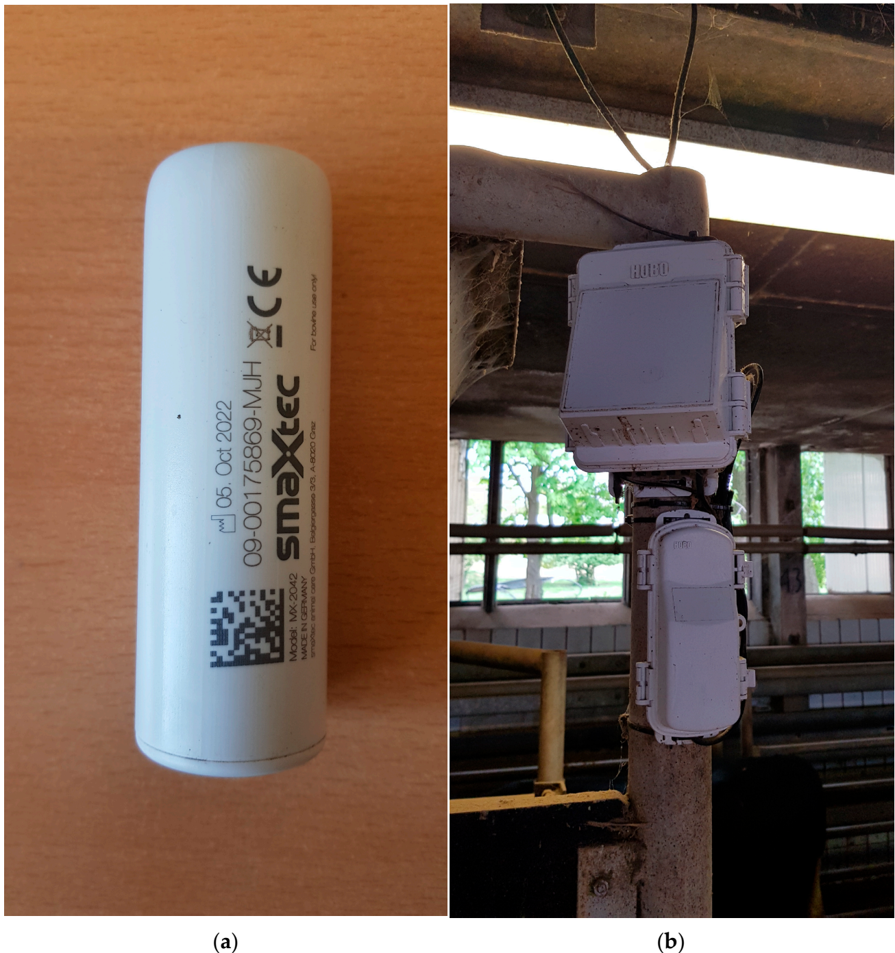
Figure 2. (a) Rumen sensor bolus. (b) Base station for Hobo Onset climate sensors (air temperature, relative humidity, solar radiation, and wind speed).
