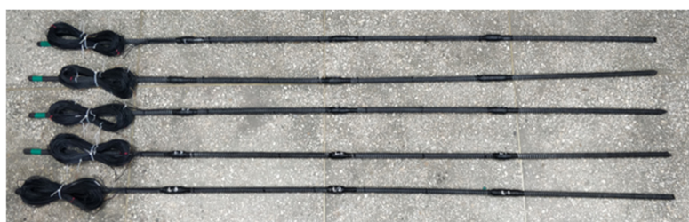
Figure 3. GFRP anchor strain sensor.
