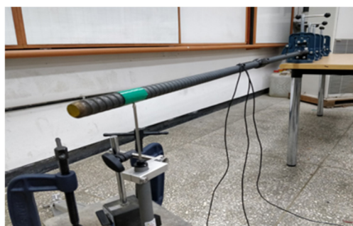
Figure 5. Sensor strain–displacement relationship measurement.
