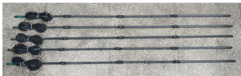
Figure 4. Steel anchor strain sensor.
