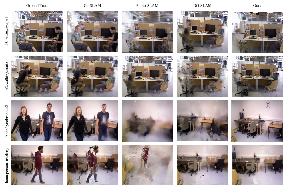
Figure 5. Qualitative comparison of rendering results on BONN RGB-D dynamic dataset. The figure illustrates that BDGS-SLAM generates fewer artifacts and maintains higher fidelity in static scene reconstruction compared to baseline methods (Photo-SLAM [2], DG-SLAM [27], Co-SLAM [30]), especially in handling complex dynamic objects.
